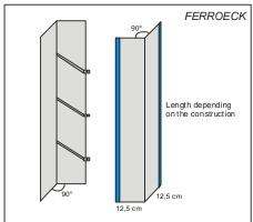
FERROSTOSS and FERROECK vertical joint elements are placed on the base plate and connected to the horizontal FERROQUELL joint metal waterstop each with two fixing clamps type VF. Furthermore the fixing devices of FERROSTOSS and FERROECK are fastened with dowels to the precast double wall.
