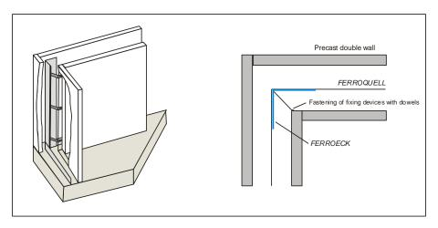
In the corner of horizontal sealing the factory-bended *FERROQUELL I* corner element (or *FERROQUELL II* corner element) should be used for an optimal connection to *FERROECK* vertical joint element.
