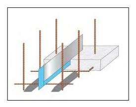
In addition to the FERROQUELL I standard there is a FERROQUELL II special version available with all-round hydrophilic rubber coating.
