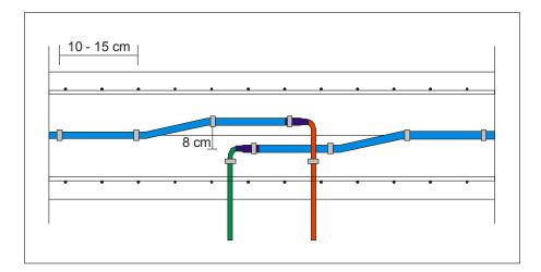
As a rule the air-bleed ends are led out of the construction at a right angle. They may be connected in protective boxes that are fixed to the reinforcement.
